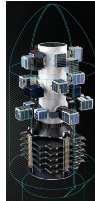
Fig. 10. CubeSats Accommodation Configuration in Fairing 6)
