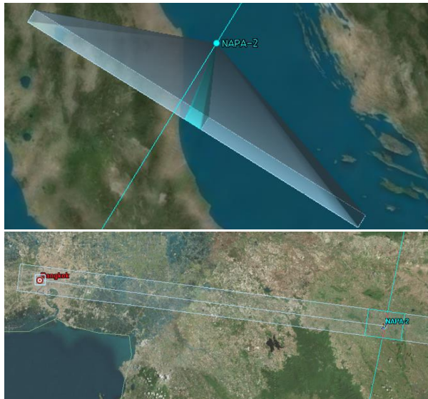
Figure 8: NAPA-2 field of view and field of regard (top) and target acquisition (bottom) in STK.
