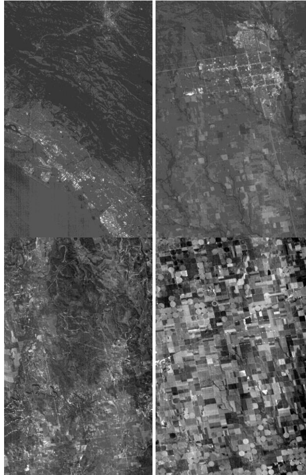
Figure 14: Different TDI levels applied, and the resulting signal level as shown in low-resolution thumbnails (manually increased brightness for comparison). From left to right: TDI 1, 2, 4, and 8.
